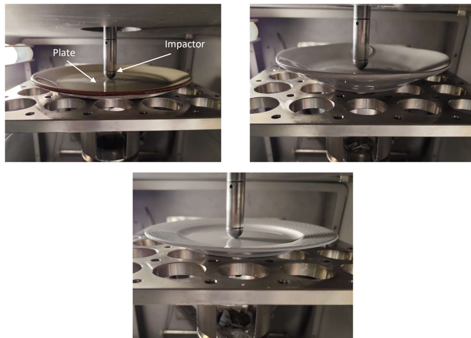
Figure 2 – Test configuration to perform multi-axial impact tests on plates
